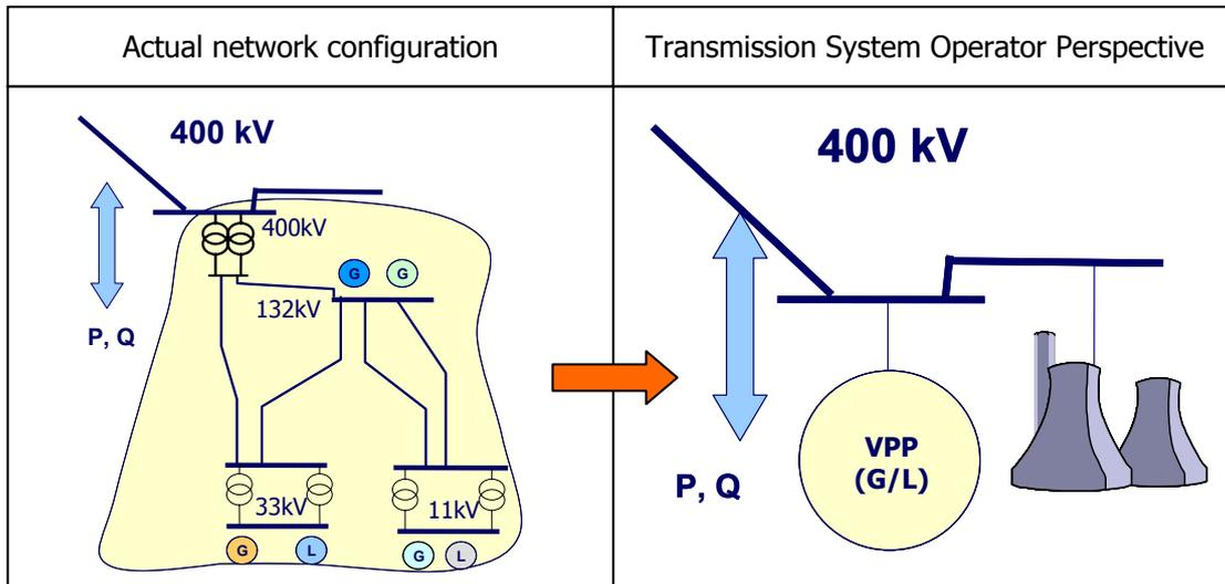
**Figure 1: Characterisation of DER as a Virtual Power Plant**
