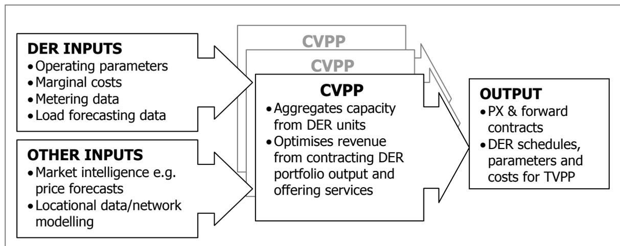
**Figure 2: Inputs to- and output from CVPP activity**
