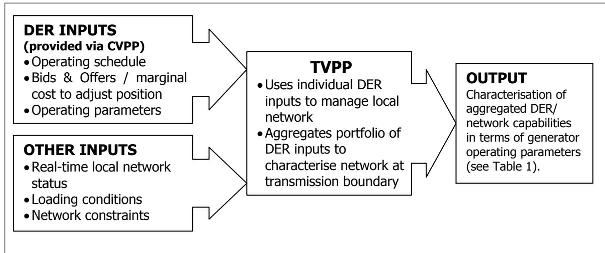
**Figure 3: Inputs to-and outputs from TVPP activity**
